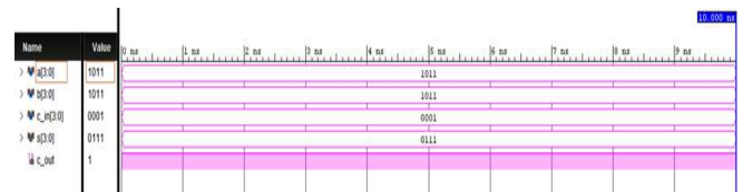
Fig. 13. Simulated output wave of proposed carry save adder where a=1011, b=1011, c in =0001
