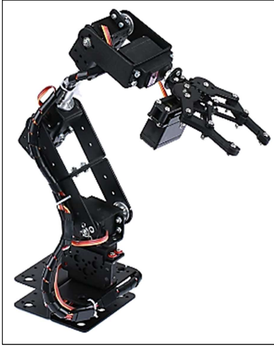
Fig. 2 Hardware setup of 6 DOF Robotic manipulator
