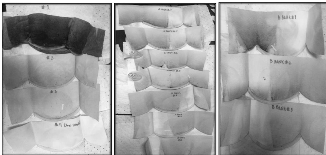
Fig. 5 Post operational flushed filter bags bottom section.
