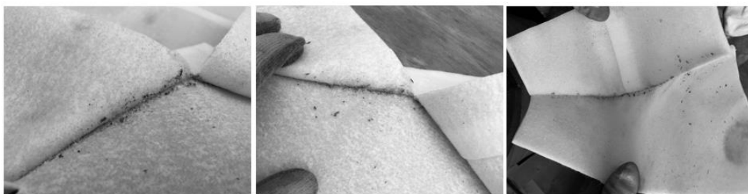
Fig. 4 Pre-start-up contamination of dry gas seal system.
