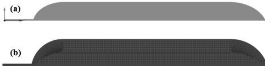
Fig. 1. a. The geometry and b. Mesh of the hydrogen storage tank.
