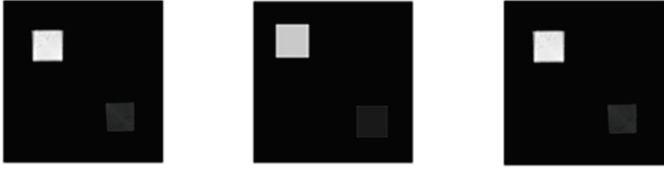
Fig.3. (a) Original image (b) Reconstructed image with infinite precision (algorithm) (c) Reconstructed image with finite precision (architecture).
